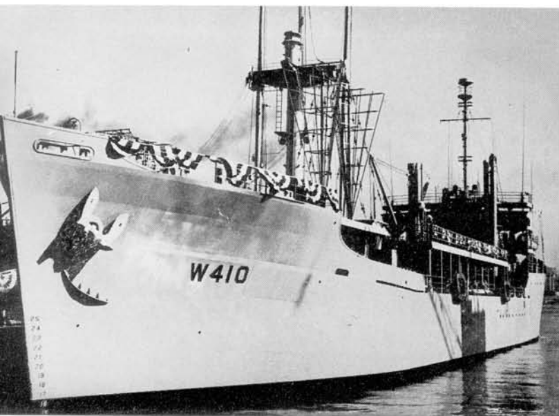
Figure 6 — The Voice of America's floating radio station "Courier." Some of the special antennae can be seen in this view. From the raised platform amidships captive barrage balloons may be released to carry antennae hundreds of feet above the ship.
